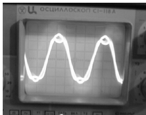
Figure 3-6. The collector-emitter and load voltages' waveforms.
